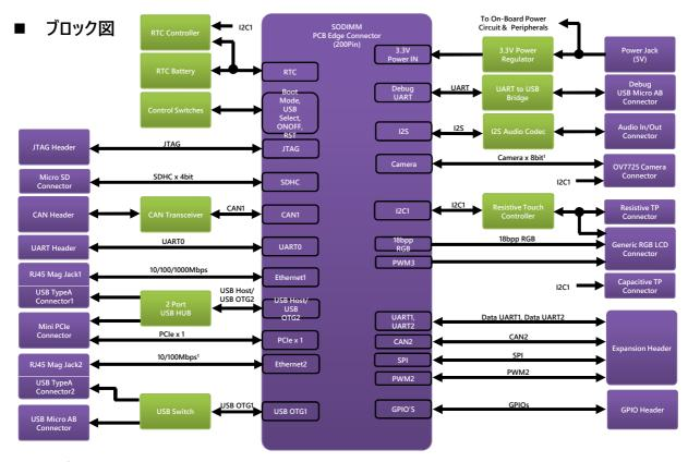
Note1: 2nd Ethernet and 8-bit camera interface is multiplexed in the RZ/G1E CPU. At a time anyone can be used. By default 8-bit camera interface is supported in the development kit.
